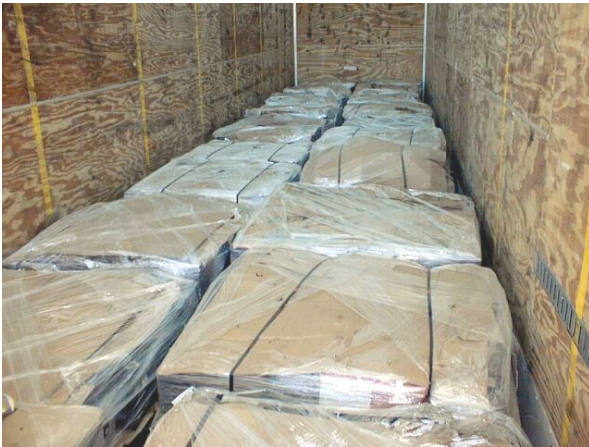
Pic. 4 – ULAB shrink-wrapped, palletized and strapped inside the truck.
