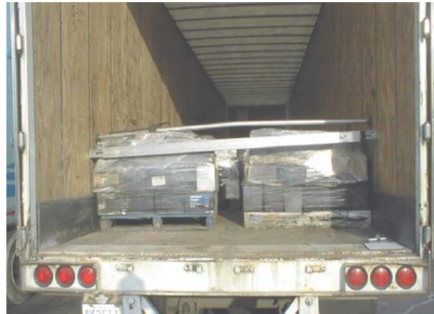
Pic. 5 – Properly blocked back row to prevent movement of the palletized ULAB
